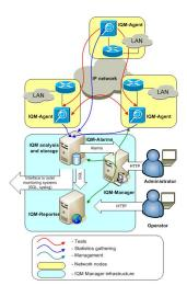
From the technical point of view, IP Quality Monitor consists of two basic elements: agents of quality parameters measurement (IQMA) and management system (IQMM).
